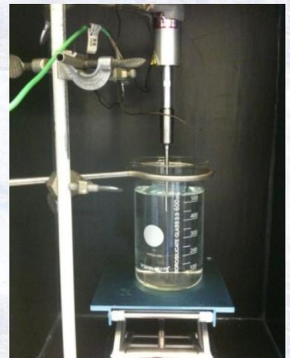
*Setup for the measurement of calorimetric curves of probe-sonication (photo kindly provided by DTU Food Denmark)*
